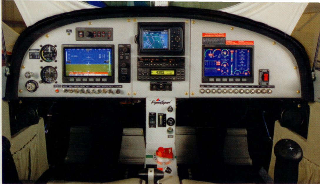
Piper will offer three versions of the PiperSport panel, including this version with a Garmin GPSMAP 496.
